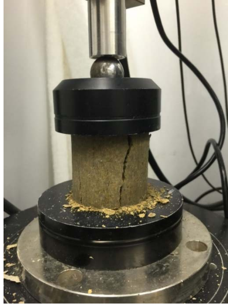
Figure 17. Specimen failure after measurement of UCS
