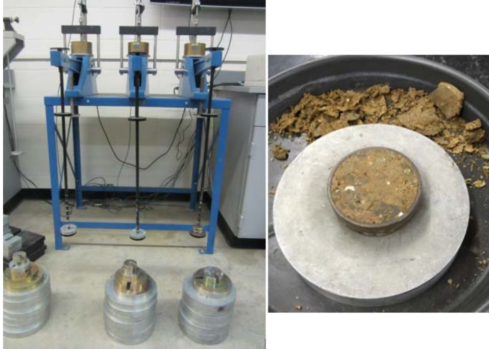
Figure 19. One-dimensional consolidation testing equipment and specimen
