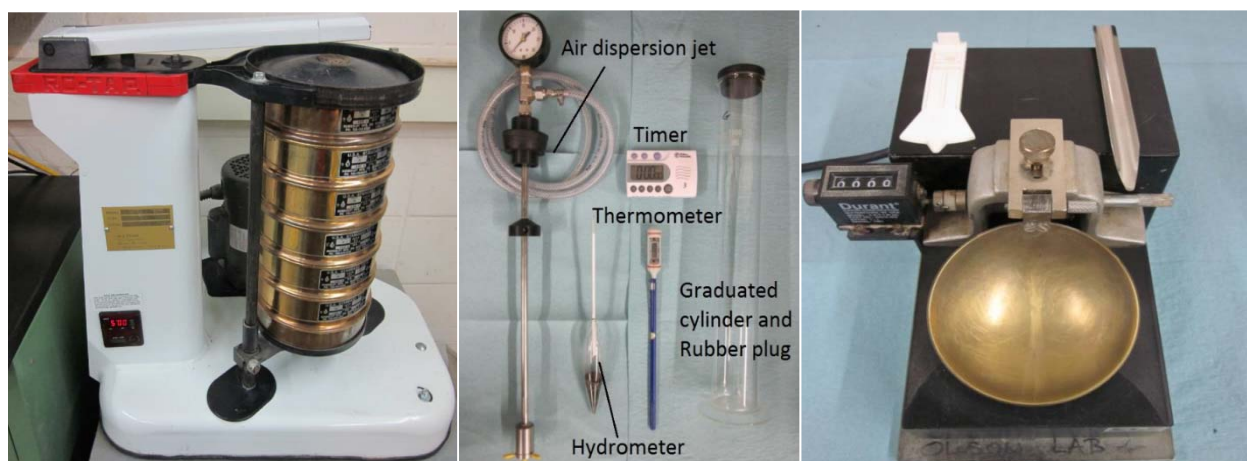
Figure 14. Soil classification equipment (left to right: sieve analysis, hydrometer test, and Atterberg limit test)
