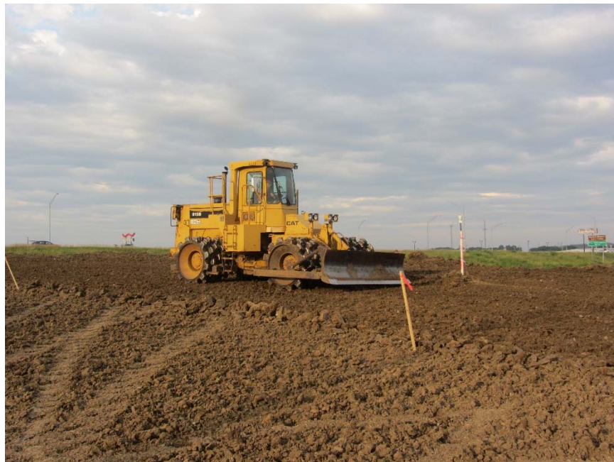
Figure 101. Pottawattamie County Project 6: Caterpillar 851B dozer with sheepfoot roller wheel used for soil compaction
